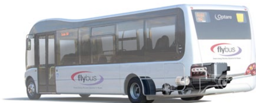
Flybus: The development of a Ricardo Kinergy flywheel energy storage device in a demonstrator vehicle based on an Optare Solo bus
