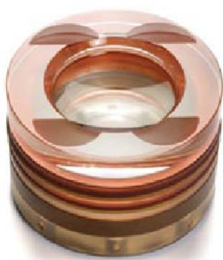
Optically accessed piston used in the Ricardo spray-guided GDI research engine;
