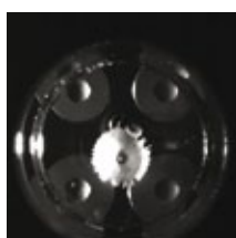
Optically accessed piston used in the Ricardo spray-guided GDI research engine;
