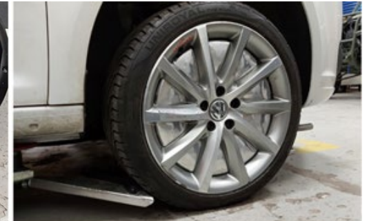
Tyre sample duct fitted behind wheel
