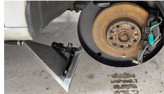
Wheel removed showing mounting of tyre sample duct, and rear of brake enclosure
